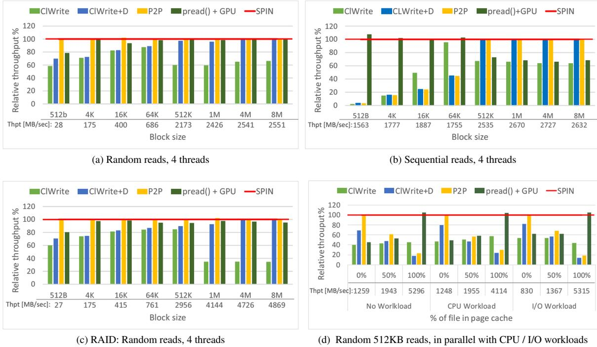
Figure 4: Threaded IO benchmarks for AMD GPUs.
